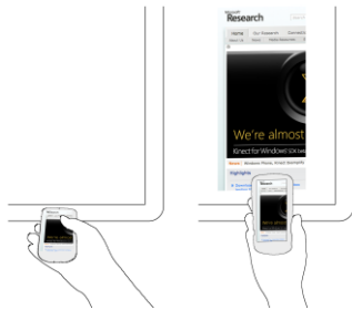
Fig. 9. User working with a mobile phone normally (left). User holds phone at arm's length and orients the phone vertically, much like holding a piece of paper up to the group. While this is maintained, the phone's contents is shared transiently with the group.
